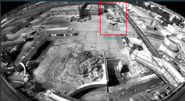
Infrared panoramic thermal imaging in false-color representation. The overall image is put together from multiple individual scans.
